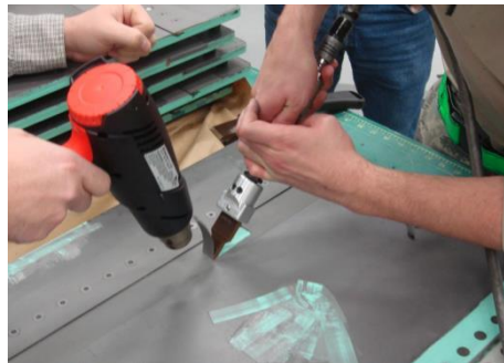
Removing Coating Material (with & without heat assistance)
