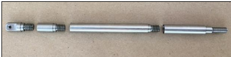
Segmented tetherable mandrel broken into a tether mounting hole (a), and a 12.7mm (0.5") (b), a 63.5 (2.50"), a 38.1 (1.50") segments
