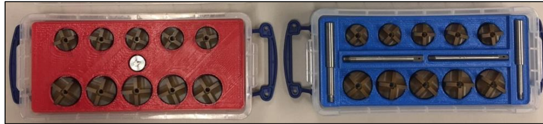
Beta kits of Torlon cutters, mandrels, and Andrews Tool Adapter
